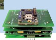
"Cookies". Modular platform for wireless sensor networks. Ability to easily combine different combinations of energy supply, types of sensors and communications.
