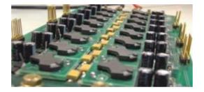
Multi-phase converters (16/36 phases) with digital controller implementation based on a FPGA.
