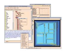
ARDID is a tool to analyze the VHDL code quality from a *hardware* point of view. It helps the designer in the VHDL-based complex systems design flow.
